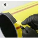
Lift the edge of the skin as shown above and peel the skin away from the core pipe.
