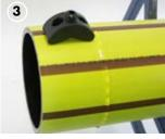
Rotate the PET<sup>TM</sup> 90° and score the external skin longitudinally towards the pipe end.
