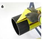
Ensure the skin is completely removed around the pipe's circumference.
