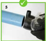
Immediately place the fitting on the pipe up to the insertion stop. Repeat steps 1 to 3 for the second pipe to be joined. Follow industry best practice when making the joint.
