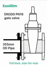
355mm EasiSlim Flange connects 355mm OD (outside diameter) PE pipe directly to a DN300 PN16 valve. A traditional 355mm PE Flange requires a DN350 PN16 valve for bolting to match.
