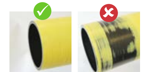
Correct pipe preparation for electrofusion
