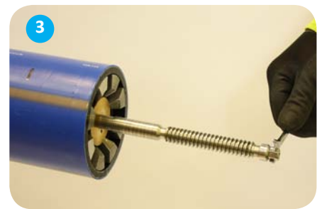
3 Using a 10mm ring spanner, secure but do not overtighten the mandrel as this will distort the pipe
