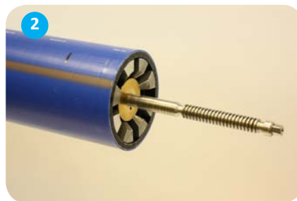
2 Select the correct size tooling for the pipe diameter. Insert the mandrel into the pipe, as shown, ensuring that the mandrel fins are equally spaced and flush with the pipe end.
