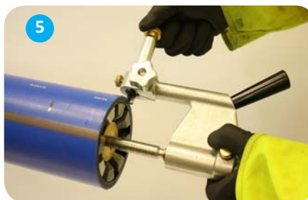
5 Depress the mandrel release button and place the body of the Puriton surface preparation tool onto the thread of the expanding plug.
