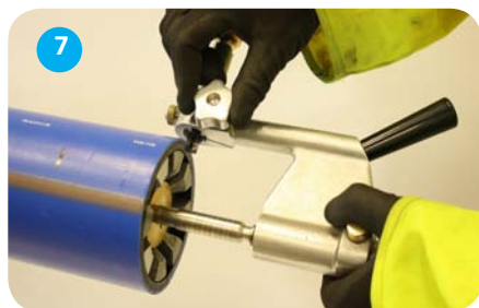
7 Tighten the locking screw and rotate the spring screw into position
