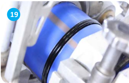
19 4. Weld cycle The final bead should be uniform in shape and correctly sized. Check the bead size using the Puriton butt-fusion gauge
