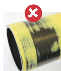
Incorrect pipe preparation for electrofusion
