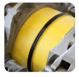
SC80 pipe is manufactured from PE80 materials and is easily identifiable by its yellow coloured outer surface.
