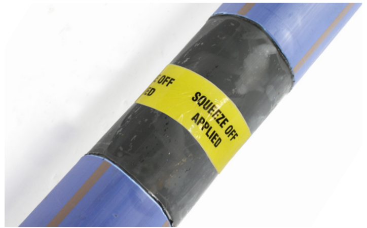
Fig. 10 'Squeeze off applied' tape on pipe following squeeze off and re-rounding
