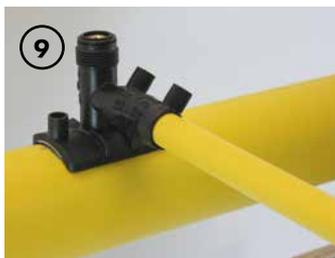
9 Prepare the outlet of the tapping tee and place the socket fitting onto the outlet. Prepare the service pipe and make the socket joint following the socket fitting jointing procedure within this brochure.
