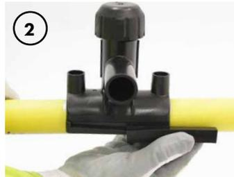
Prepare the pipe surface following the 'Top loading tapping tee jointing guidance' within this brochure. Place the fitting on the pipe. Position and slide the underpart in the groove of the upper saddle as shown.
