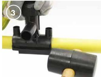
Hold the upper saddle firmly while tapping the underpart with a suitable soft-blow hammer to fully engage the underpart.
